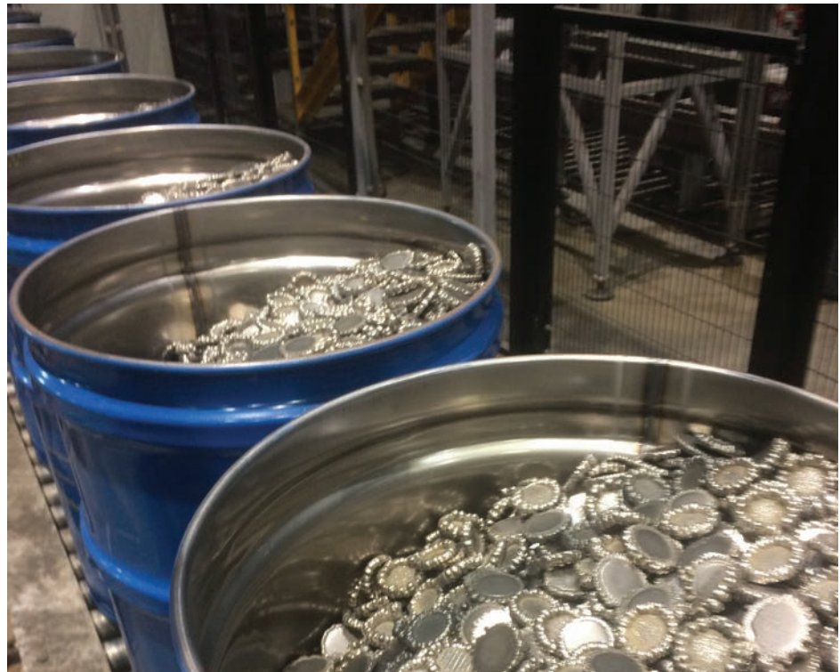
Cobalt rounds from the Voisey's Bay Long Harbour processing plant which became operational in 2014, and has total production capacity of 50,000 tonnes of nickel per annum. In addition to nickel and copper, the Long Harbour plant produces high purity cobalt rounds from Voisey's Bay concentrate. Credit: Vale
